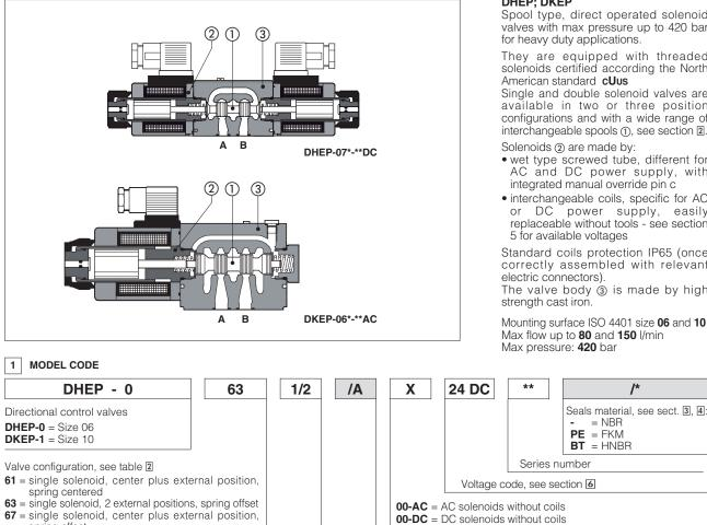
75= double solenoid, 2 external positions, with detent
